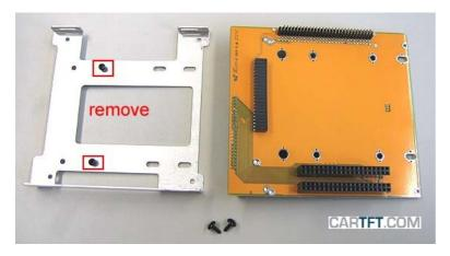
The HDD gets mounted onto the Drive Adapter:
