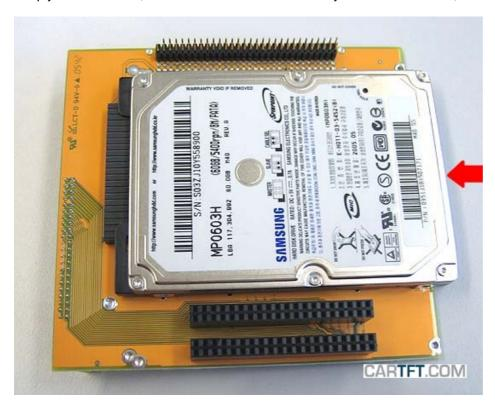
Flip over the Drive Adapter, for installing and tightening the CD-ROM Bracket, Insulate Pad and the HDD with screws.
