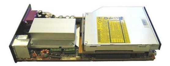
Before the motherboard gets slid in the case again, the fake-drive blend has to be removed of the case, so that the correct CD/DVD-ROM can be used.
