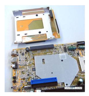
The Drive Adapter gets turned over, for removing the little, black plastic fastener:
