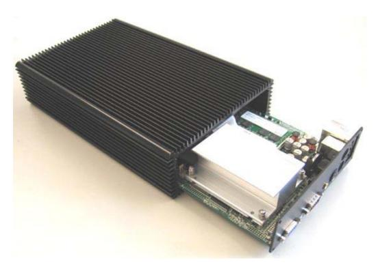
Finally the motherboard gets screwed at the enclosure. Finished – The CALUCORE-M is assembled.
