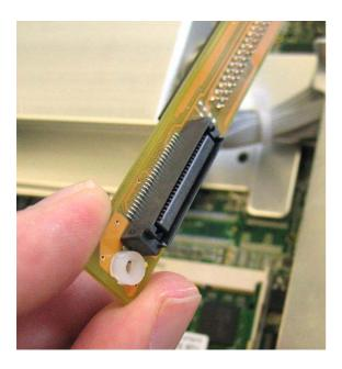
After that the CD/DVD drive can be connected to the slimline adapter and it can be screwed with the long screws of the adapter:
