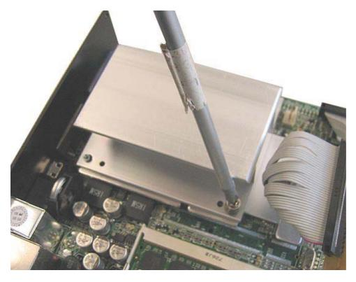
We go on with tightening the mounting unit to its previous place again.
