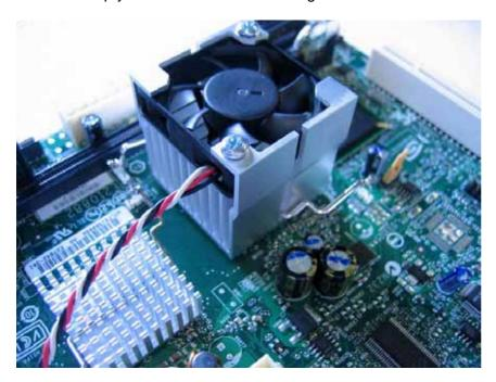
Therefor press down the metal holding clamp and then rotate the heatsink carefully.
