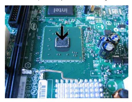
Remove the protection foil from the new heatsink and place it with soft pressure on the chipset. Take care of positioning in a way so you can insert the metal holding clamp later on (see pictures below)
