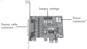
Figure 1: CyberSerial 4S PCIe Board Layout
