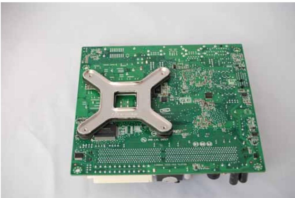
Turn around the mainboard now, be careful to hold the mounting cross and push it slightly so it does not slide off.
