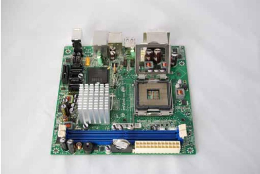
Place the corresponding CPU in the for this purpose provided recess (it will only fit in one direction).
