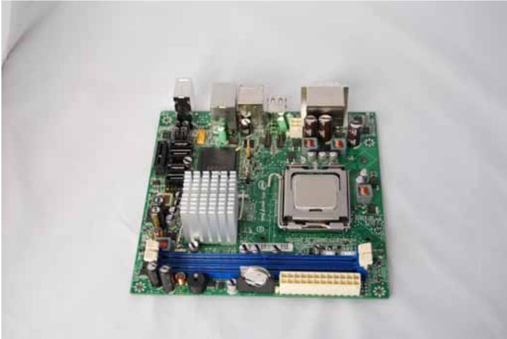
Please turn the mainboard around carefully. You need to be very careful when mounting the heatsink/fan with the mounting cross, because the chipset (see picture) can easily be damaged.
