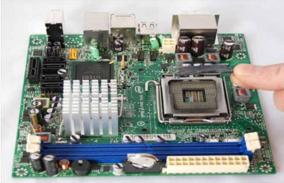
Now press the bolting of the socket outward and upward.
